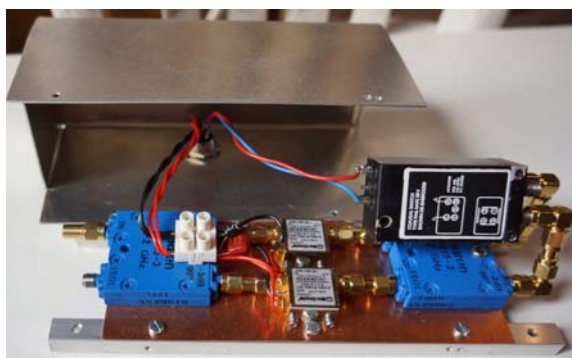
Figure 2a Preamplifier/Switch Unit
