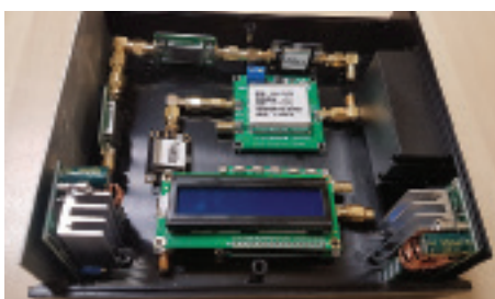
PHOTO 2: Early-on in the layout process for a much more compact, cased prototype. Solid SMA adapters are used instead of SMA-SMA leads.
