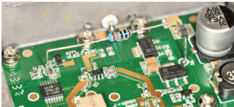
PHOTO 5: Adding a 100k resistor inside the power amplifier from TP2 to TP4 to defeat the VOX. Most other comparable types of Wi-Fi ‘booster’ can be modified in a similar fashion.
