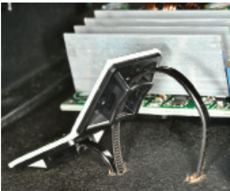
PHOTO 3: Using cable tie bases 'in reverse' to mount the PSU boards (one with integral heatsink seen here behind the cable tie base).
