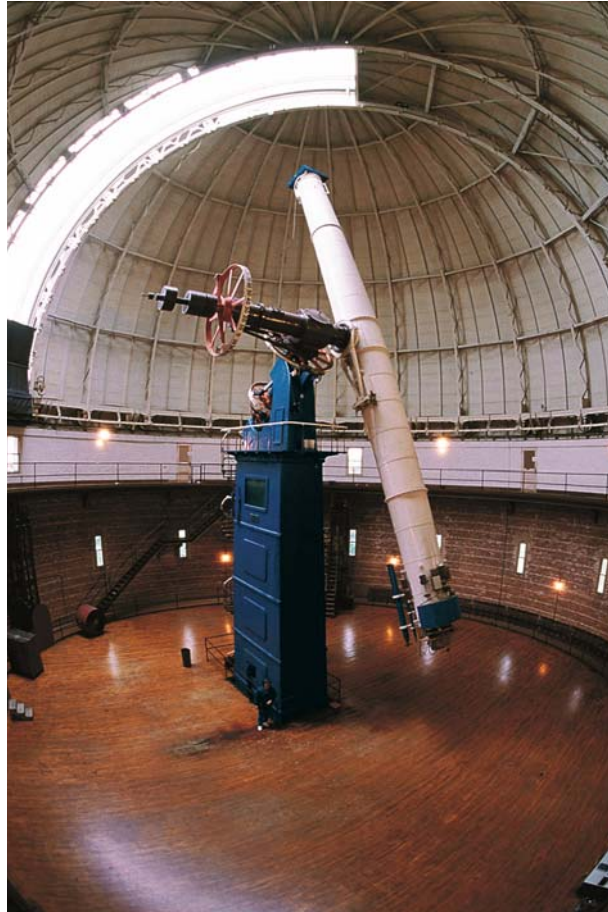
Figure 1.4. The great 40-inch Clark refractor of Yerkes Observatory, located at William's Bay, Wisconsin. Long used for both visual and photographic studies of double stars, it is typical of the long-focus refractors traditionally employed in such work. The tube of this mammoth "celestial cannon" spans 65 feet in length, and it remains the largest lens-type telescope in the world today. Courtesy Sky & Telescope and P. K. Chen.
