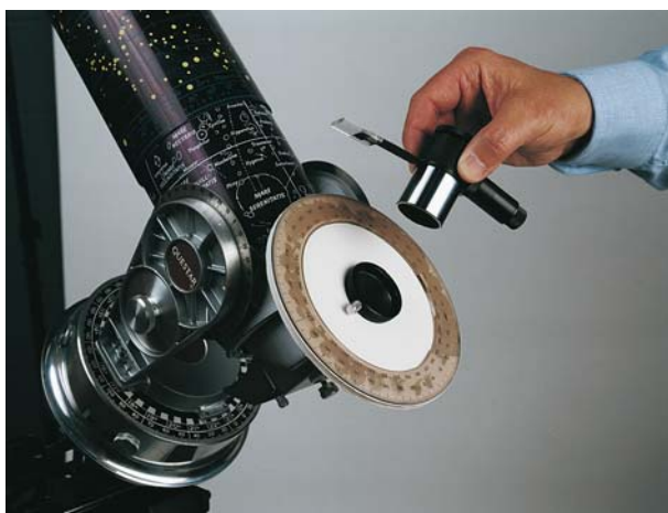
Figure 5.6. A reticle-eyepiece micrometer assembled by American observer, Ronald Tanguay, and mounted on his 3.5-inch (90 mm) Maksutov-Cassegrain telescope. A protractor scale and pointer were added to a commercially available reticle guiding eyepiece, as seen in these two views. Using this simple device, he has made numerous double star measurements of high precision with this small-aperture instrument. Courtesy Sky & Telescope .
