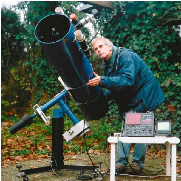
Figure 5.8. The video-imaging setup of German amateur Rainer Anton on his homemade 10-inch Newtonian reflector. An inexpensive commercial black and white camera is used to shoot tricolor images through red, green and blue filters. The camera head and filter wheel is seen here attached to the telescope's 2-inch focuser. A camera controller and digital video recorder are seen in the foreground. Courtesy Rainer Anton.
