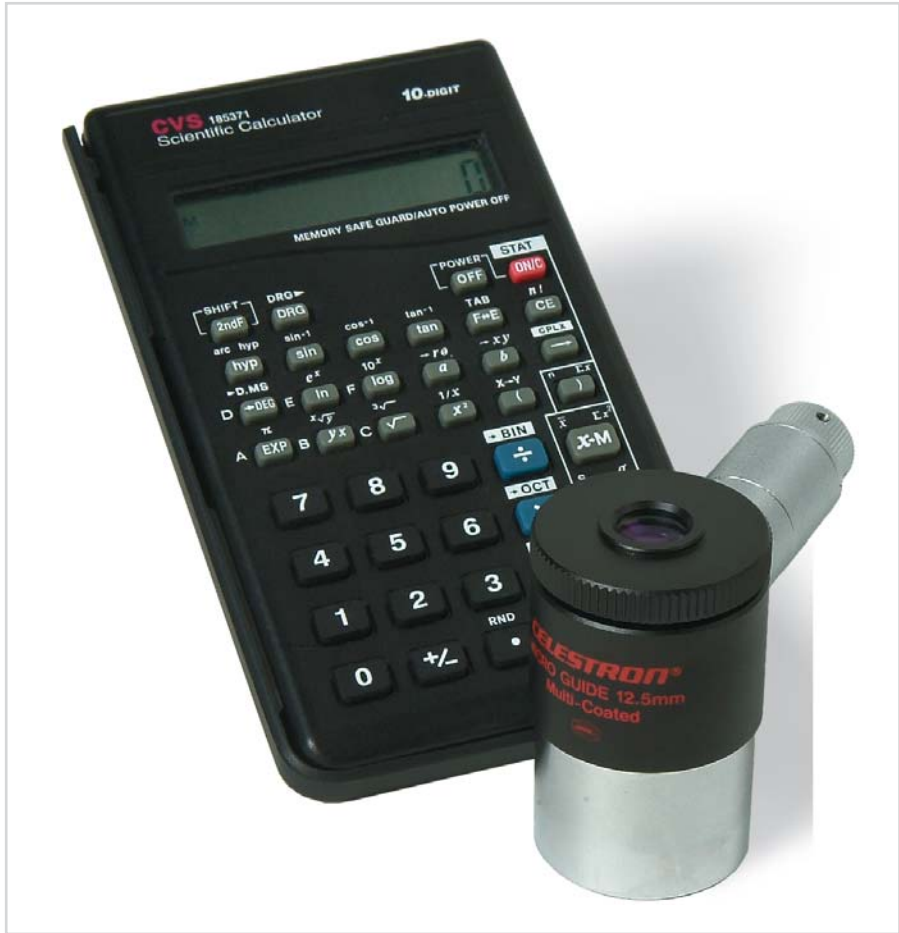
Figure 6.7. With these two simple, commercially available tools any amateur having a steady, equatorially mounted telescope with good optics can do valuable double star work. Shown is an illuminated reticle eyepiece for making the actual measurements and an ordinary scientific calculator for reducing the observations. Another reticle eyepiece micrometer appears as Fig. 5.6 in the previous chapter. Courtesy Sky & Telescope .
