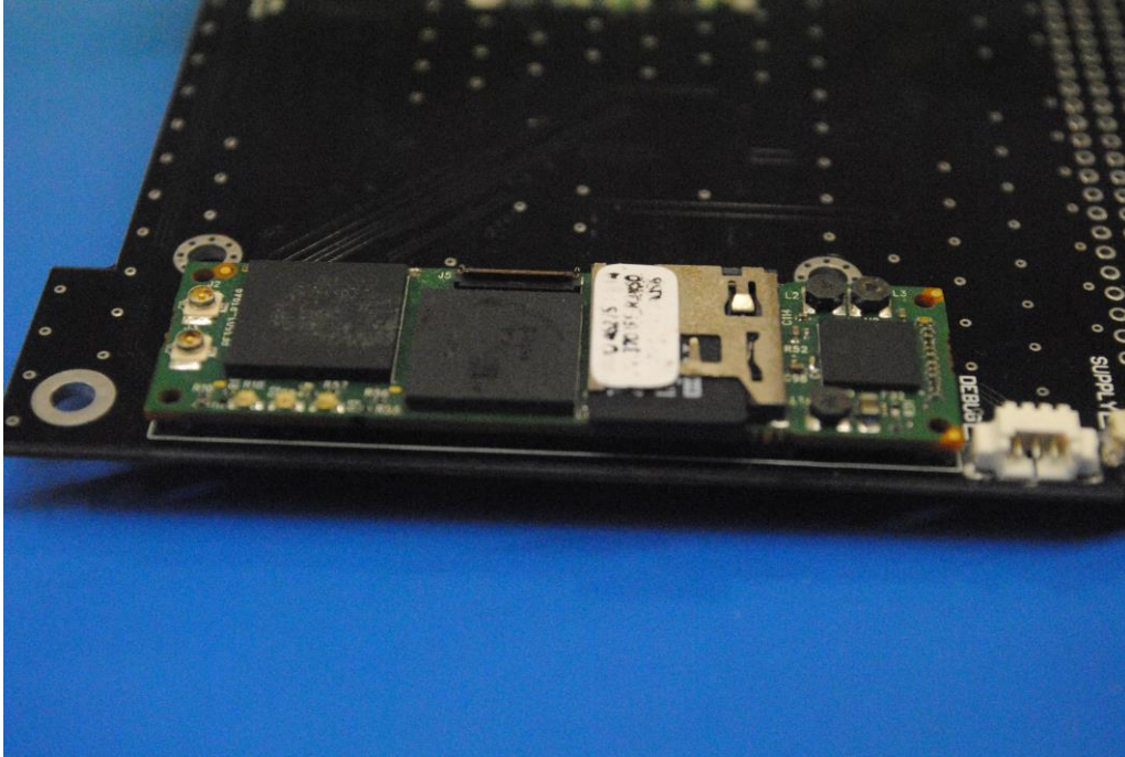
Figure J-5: Overo Ironstorm-P connected
