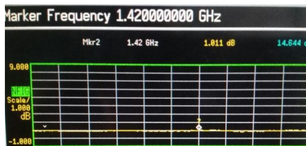
Figure 4-13: Characterization of the SPF-5043Z transistor acting as an ACL
