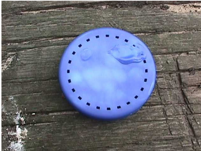
LNB protection sunburned
